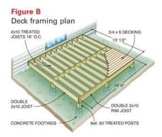
DRAWINGS – These should be drawn to scale with detailed dimensions, framing details and footing/foundation details. A lot survey should be Included with the plans to detail the location, lot lines, and easements
